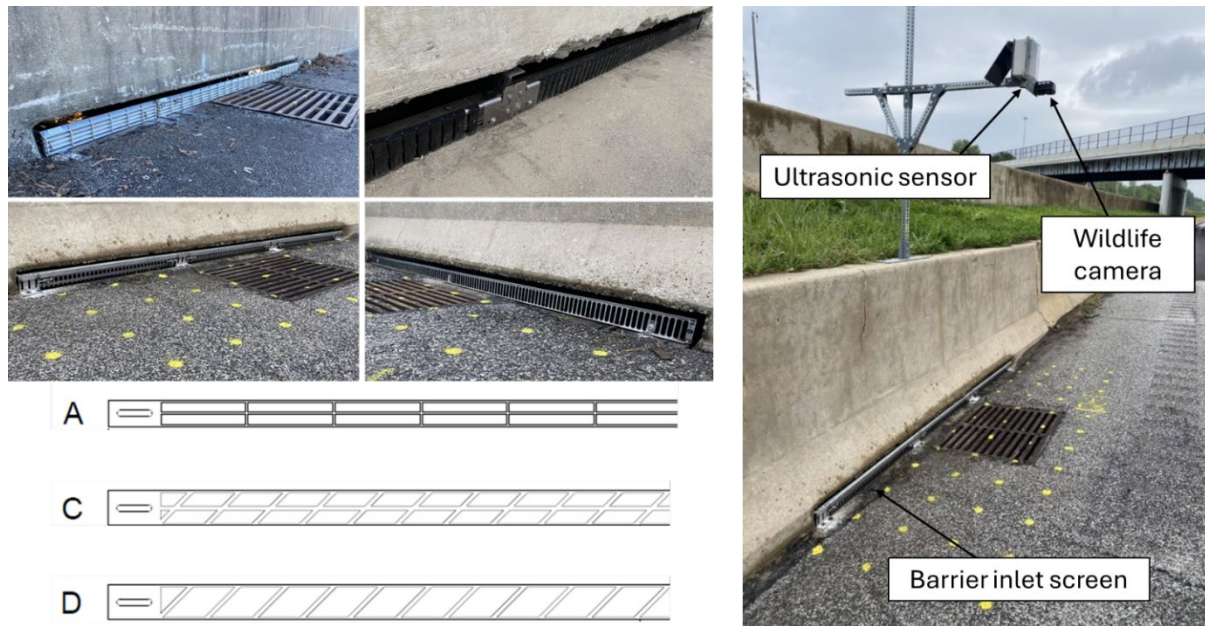
Figure 1: Photos of four proprietary barrier inlet screens (upper left), design of non-proprietary screens (lower left), and field monitoring apparatus designed for real-time monitoring of roadside ponding depth (right).
